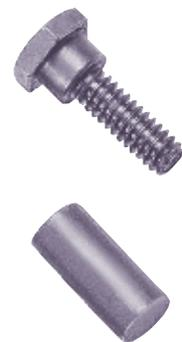
**Fig. 9** The shoulder on this part is the same size as the wire diameter, while the shank was extruded and the head upset and trimmed.
