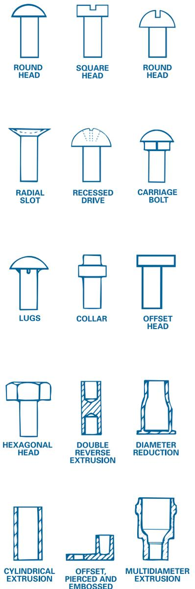
**Fig. 10** A wide range of designs are possible for cold headed parts.
