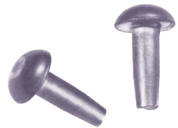
**Fig. 7** Simple upsetting was used for the screw blank on the left, while contained extrusion was used to form the part on the right.
