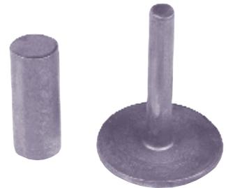
**Fig. 8** The shank of this part was trap extruded, and the head trapped and upset to produce the exaggerated head to shank ratio.
