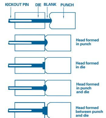
**Fig. 3** The upset of fastener heads is accomplished using one of these four methods:
