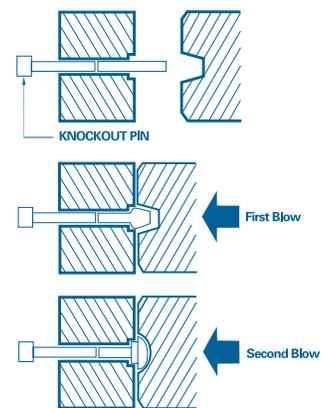
**Fig. 4** The knockout (or kickout) pin plays an important role in solid die heading. The pin acts as a blank support and also ejects finished parts.
