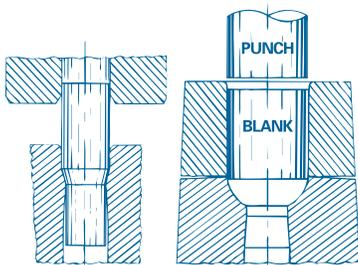
**Fig. 6** Extrusion is either open (left) in which the blank is forced under pressure into a smaller diameter die hole, or it is trapped where the blank is totally confined within the die prior to extrusion (right). Trapped extrusion permits reductions in area of up to 75 percent, while open extrusion allows only 30 percent area reduction in one blow.
