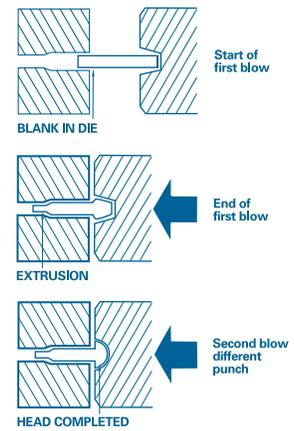
**Fig. 2** The typical one-die, two-punch method is common in producing headed parts, especially fasteners. The first blow combines partial head upset (coning) with shank extrusion, while the second blow finishes head shape.
