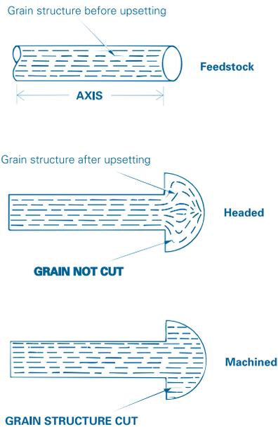
**Fig. 11** Heading improves the finished part's grain structure by making it conform to the flow of the design. The machined fastener on the bottom indicates how metallurgical structure is weakened by operations that cut across flow lines.
