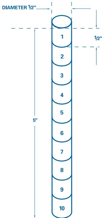
**Fig. 5** This simplified diagram shows how diameters of wire are calculated to determine upsetting limits.
